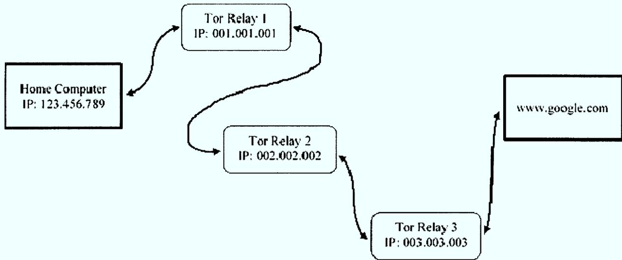
In this illustration of a Tor network connection, the website www.google.com cannot see the home computer IP address (123.456.789); instead it only sees the IP address of the device it is directly connected to, the third (or “exit”) Tor relay, with IP address 003.003.003, which IP address cannot be traced back to the home computer user.
