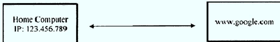
In this illustration of a standard internet connection, the website [www.google.com](http://www.google.com) can see the home computer IP address (123.456.789) and, of course, the user of the home computer knew the URL, and therefore the IP address, of [www.google.com](http://www.google.com), which the user had to type into his browser to connect to the website in the first place. Thus, each users’ IP address is known to the other, and the owner and location of both can later be traced.
