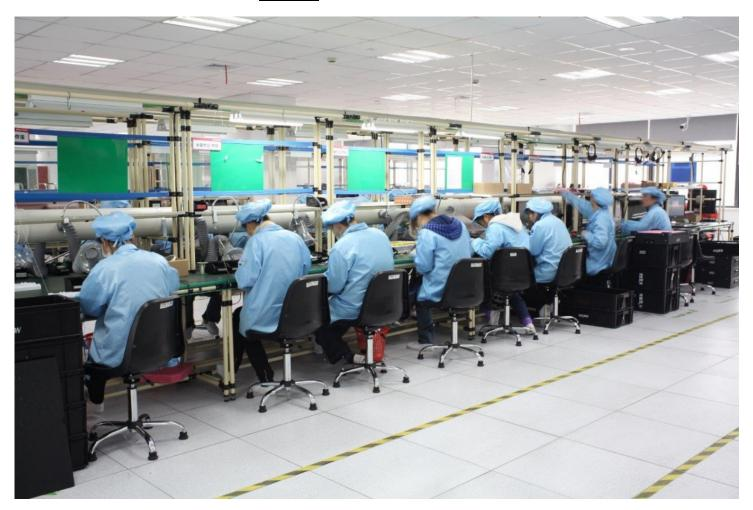
This area is running a single 8-10 hour shift and has a daily capacity of 18,000 IP cameras. The lines are building fixed domes, box cameras, transport cameras, bullet cameras and more. There's a lot of assembly work with cameras – the lenses, housings, dome bubbles, terminations and all the rest have to be hand-built.
